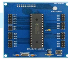
CPU : PIC16F874/877 PIC18F452
