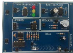
Digital Temperature, RTC EEPROM, SPEAKER, IrDA
