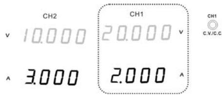
Master (CH1) voltage level: CH1 meter reading shows the output voltage. In the above case, 20.0V.
