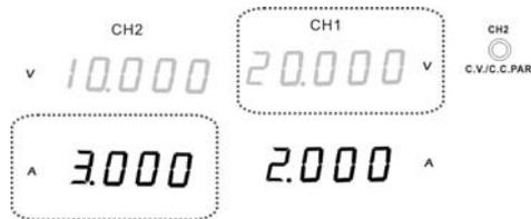
Master (CH1) voltage level: CH1 meter reading shows the output voltage. In the above case, 20.0V.
